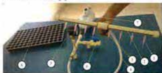
1, Mouthpiece; 2, seeder pipe; 3, pressure cut-off device; 4, flexible hose pipe; 5, pressure dial gauge; 6, pressure control valve; 7, suction unit; 8, protray
